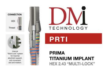
PRTIself-tapping screw titanium dental implant, conical shape, with varying thread, with an internal connection hex. Implants are made of medical titanium alloy Ti6Al4V ASTM 136. The outer surface of the implant has a double treatment (sand blasting and acid treatment). The texture of the outer surface of the implant has micro pores of 1-4 microns in size and
